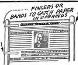
Gripper fingers shown left and right are Auxiliary Horizontal Gripper Fingers, made to hold the paper by reaching in between lines where type form is too big to allow using press grippers, except outside of form.
