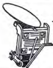
LARGE "M" LOCKED IN EACH CORNER OF CHASE TO TEST IMPRESSION.
